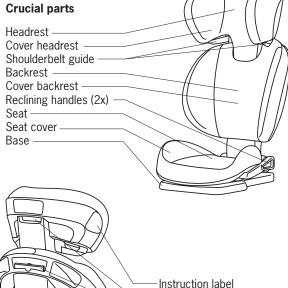
Carrying handle Storage user manual Height adjusting lever (2x) Forward-facing belt installation
